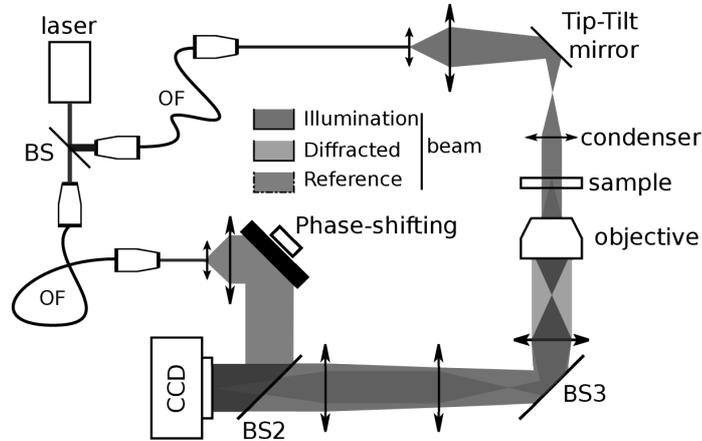
Figure 2. TDM hardware components schematic.
