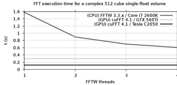
Figure 8. 3D FFT computing time for a  $512^3$  complex volume of single-floats, performed in FFTW 3.3 CPU library and cuFFT 4.1 GPU library. FFTW computations were performed with pre-optimizations in exhaustive mode.
