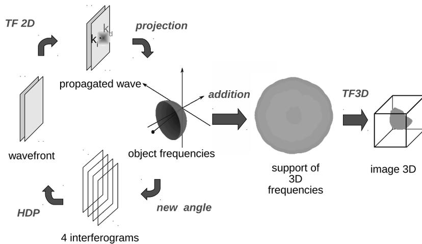
Figure 3. Image reconstruction from acquired interferograms to a complex 3D image of the specimen.
