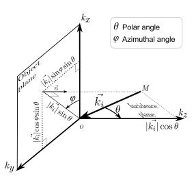
Fig. 4. Notations and coordinate system. In this work, the angular scanning is performed at a fixed polar angle so that  $k_{iz}$  remains constant.
