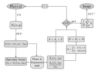
Fig. 1. 2D synthesis process for amplitude imaging. *H*, hologram; *E*, complex optical field; *S*, spectrum in original support  $\Gamma$ .  $\hat{S}$ , normalized spectrum in synthesized support  $\Gamma'$ . M, redundancy map used to average the merged data; *i*, index of the illumination angle.
