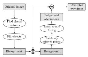
Fig. 5. Process for automatic aberration removal.
