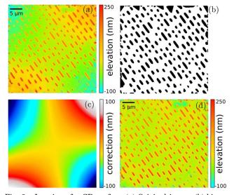
Fig. 6. Imaging of a CD surface. (a) Original image, (b) binary object mask, (c) computed correction map, and (d) final corrected phase image.
