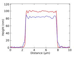
Fig. 9. Measurements of the VLSI target step height. Bluedashed curve: the unwrapping process failed and the height measurement is underestimated. Red curve: correct value estimated by double measurement.
