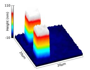
Fig. 8. VLSI test pattern of 100 nm height imaged with circular scanning  $(|k_{iz}| = \text{constant}, \theta = 40^{\circ})$ .
