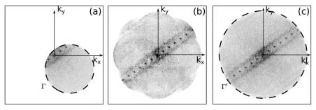
Fig. 2. Spectrum modulus of a CD reconstructed with (a) one illumination ( $\Gamma$  support). (b) Eight illuminations with bandpass enlargement and (c) 100 illuminations with noise averaging ( $\Gamma$ ' support).
